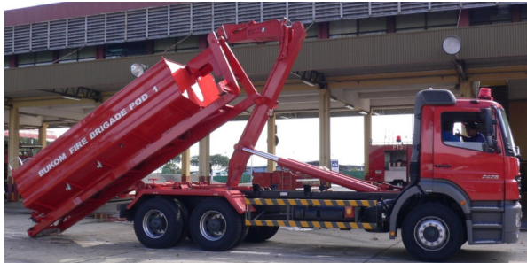
3% AFFF/AR foam from mobile foam pod
